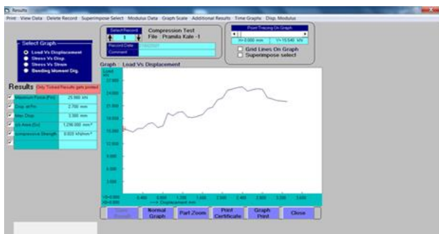
Fig. 6 Graph of maximum compressive force of Tackletic Basal
