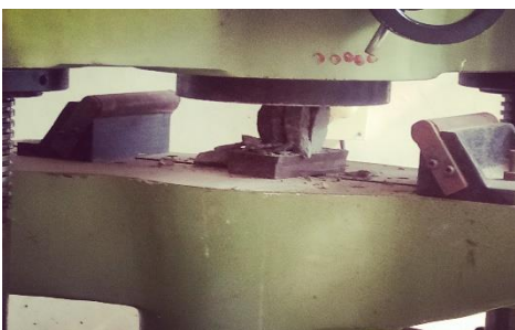
Fig.3: Rock strength testing on UTM .
